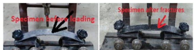
Figure 5. Specimen loaded in fatigue (cyclic) stress.
