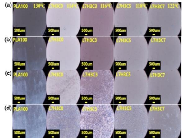
**Figure 2.** POM photomicrographs of PLA and compatibilized PLA/PHA (70/30) blends: at (a) initial crystallization temperature; (b) 120 °C; (c) 110 °C; (d) 100 °C.
