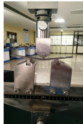
Figure 7. The experimental setup and loading arrangement of specimens for the flexural test.
