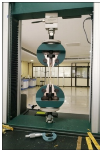
Figure 4. The loading arrangement of the test sample in the tensile test machine.
