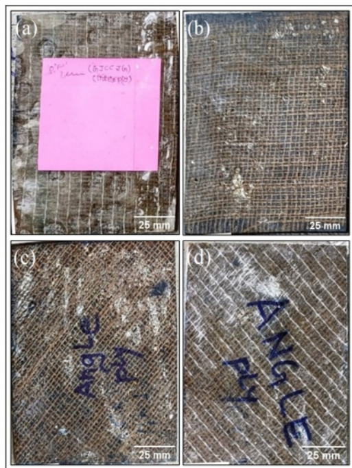
Figure 3. (a) GJC0 (Inter-ply); (b) JCG0 (Inter-ply); (c) JCG45 (Angle-ply); (d) GJC45 (Angle-ply) laminate composites.
