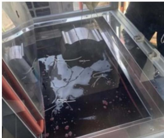
**Figure 4.** Stator in heated AFT for oil resistance evaluation.
