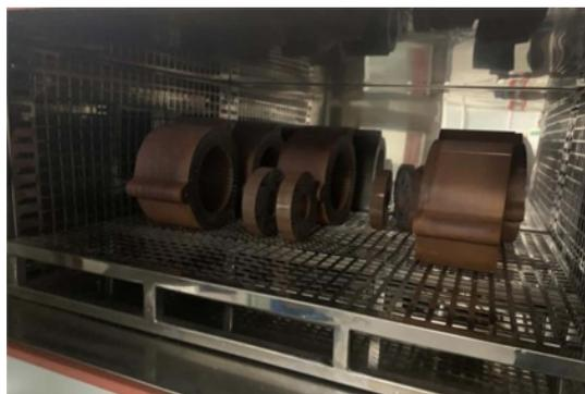
**Figure 3.** Bonding cores in the oven for high temperature treatment of thermal shock test.
