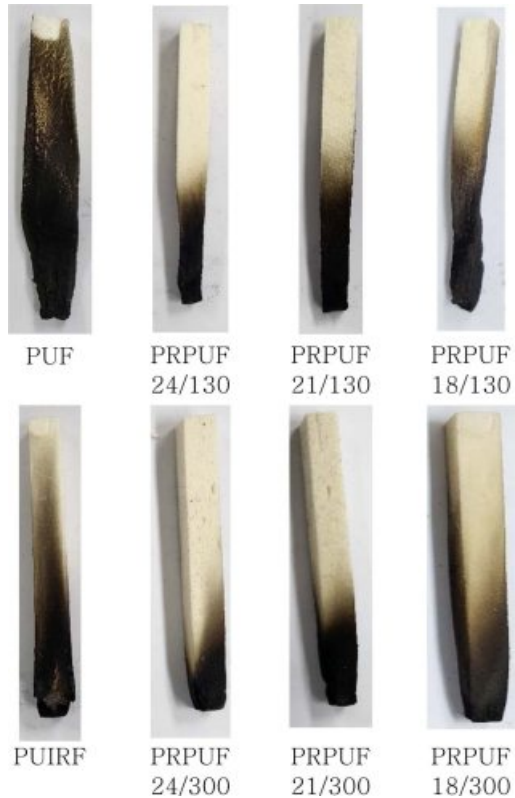
Figure 9. Results of UL94 V test of Polyurethane foams with different NCO% and NCO index.
