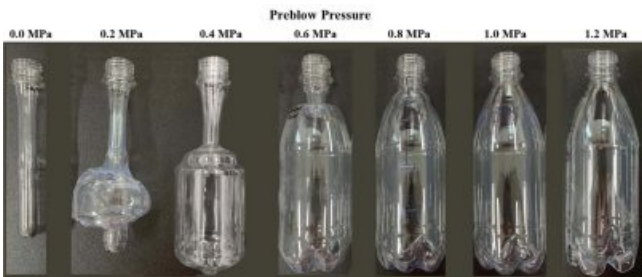
Figure 10. Blowing phenomena by preblow pressure.
