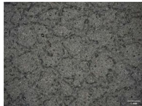
Figure 5. Specimen for testing (TPU PSM, leather grain).
