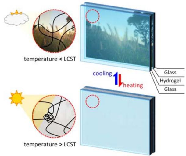
**Figure 1.** Illustration of the adaptive solar control for the smart windows fabricated with thermotropic hydrogels.
