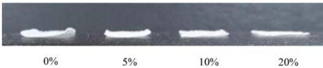
**Figure 12.** Sintered single layer of SLS printed PP powder and SLS PP powder with PP/PE copolymer.
