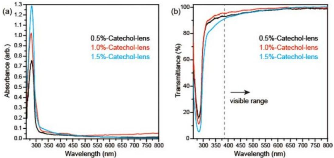
Figure 2. (a) Absorption; (b) transmittance spectra of catechol-lenses.
