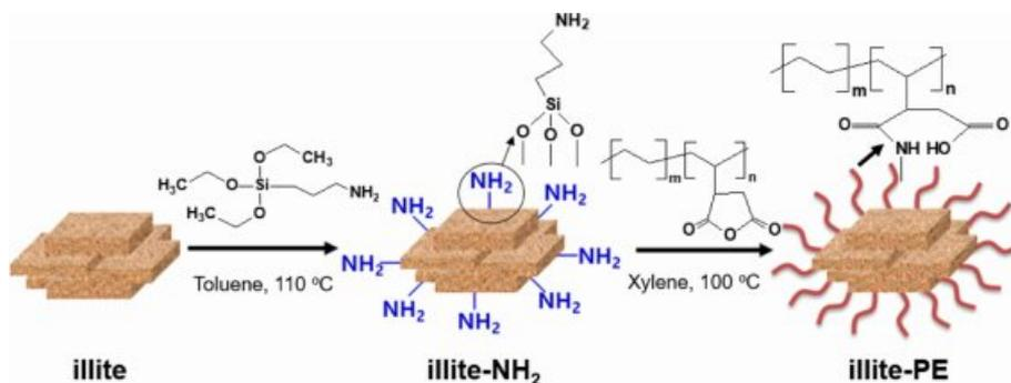
Figure 1. Illustration of the surface grafting of PE on illite surfaces.
