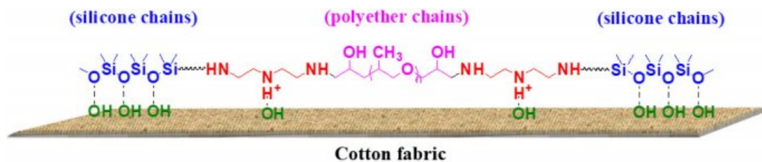
Figure 6. Adsorption model of ATSO-PDE on cotton fiber.
