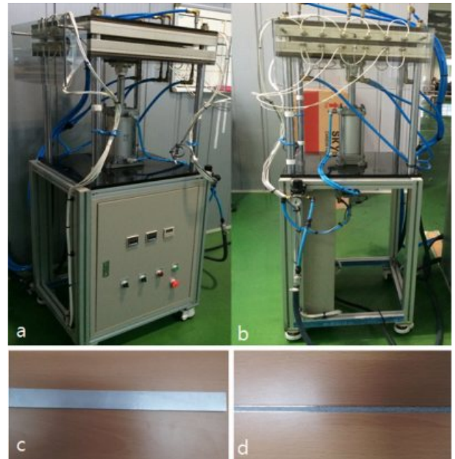
Figure 2. Photographic images of hot press (a: side view, b: front view) and produced FML specimen (c: top view, d: side view; dimension: 30 cm×2.5 cm).
