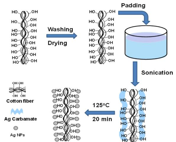
**Figure 2.** Illustration of the processes involved in the coating of cotton fibers with AgNPs using silver isopropylcarbamate.
