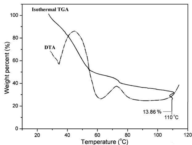
**Figure 1.** DSC and TGA thermograms of Ag-IPCB complex solution using isothermal aging up to 110 °C.
