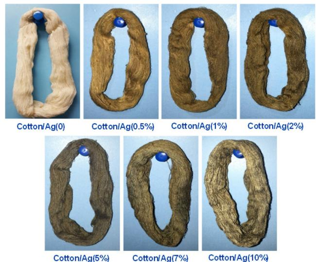
**Figure 3.** Optical images of cotton threads prepared with different loadings of AgNPs.
