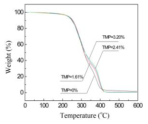
Figure 5. TG curves of the PU films with different contents of TMP.
