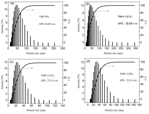
Figure 2. Particle size distributions of PU dispersions with different contents of TMP: (a) TMP=0%; (b) TMP=1.61%; (c) TMP=2.41%; (d) TMP=3.20%.
