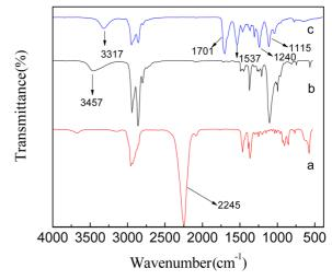
Figure 1. FTIR spectra of IPDI (a); PTMG1000 (b); PU (c).
