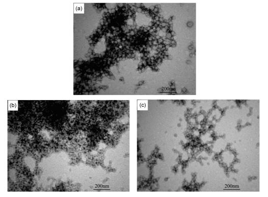
Figure 4. TEM photograph of PU dispersions with different contents of TMP: (a) TMP=0%; (b) TMP=2.41%; (c) TMP=3.20%.
