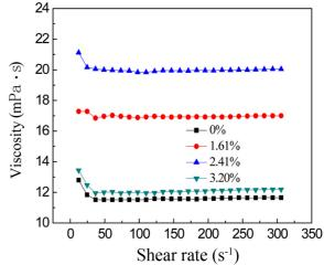
**Figure 3.** Viscosities of PU dispersions with different contents of TMP.
