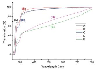
**Figure 7.** Optical transmittance of the hydrogel membranes containing  $\beta$ -CD/ $\alpha$ -tocopherol complex: (A) 0.001 g; (B) 0.005 g; (C) 0.010 g; (D) 0.05 g; (E) 0.1 g in 12 mL of monomer solution.
