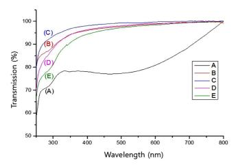
**Figure 4.** Optical transmittance of soft contact lenses prepared using different cross-linkers. The concentration of cross-linkers: (A) without cross-linker; (B) 0.1 M EADA; (C) 0.1 M EGDMA; (D) 0.1 M EADA+0.1 M EGDMA; (E) 1 M EADA.
