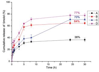
**Figure 5.** Cumulative amount of timolol maleate released from the hydrogel membranes as function of incubation time. The concentration of cross-linkers: (A) without cross-linker; (B) 0.1 M EADA; (C) 0.1 M EGDMA; (D) 0.1 M EADA+0.1 M EGDMA.
