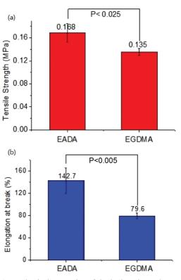
**Figure 3.** Mechanical properties of the hydrogel membranes made from two types of cross-linker: (a) tensile strength; (b) elongation at break.
