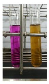
**Figure 2.** Images of a 0.02 M KMnO<sub>4</sub> solution before (pink, left) and after (brown, right) added with 0.01 M EADA solution.
