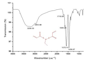
Figure 1. FTIR spectrum of the cross-linker, EADA.
