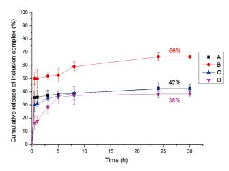
**Figure 8.** Cumulative release of  $\alpha$ -tocopherol from soft contact lenses containing the  $\beta$ -CD inclusion complex. The concentration of cross-linker: (A) without cross-linker; (B) 0.1 M EADA; (C) 0.1 M EGDMA; (D) 0.1 M EADA+0.1 M EGDMA.
