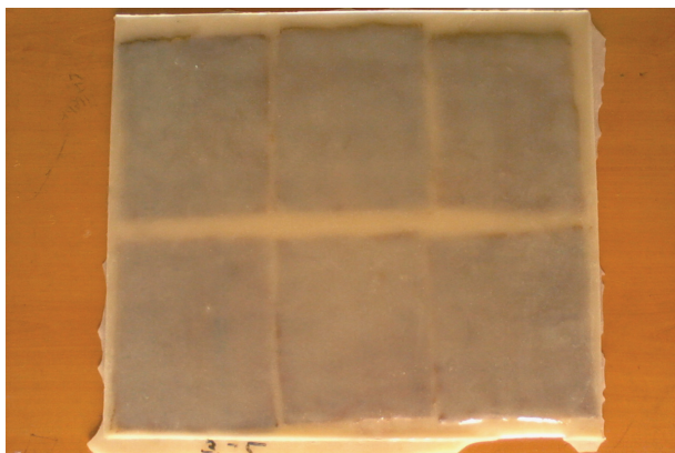
Figure 2. Fabricated HFRP specimen.
