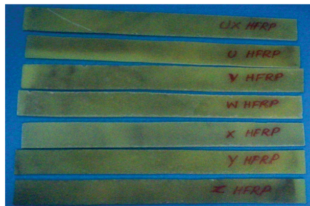
Figure 3. Specimens for tensile test.
