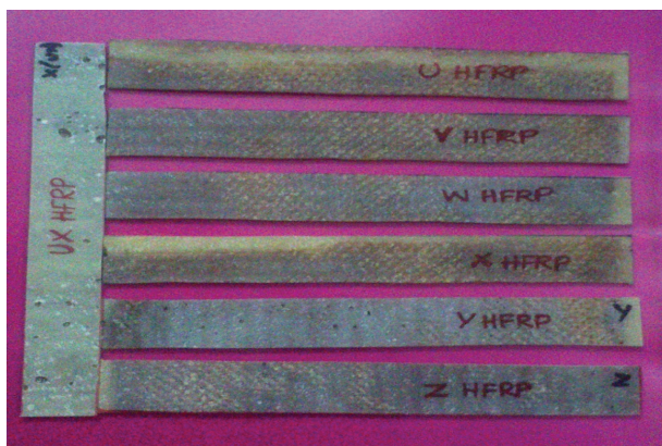
Figure 4. Specimens for flexural test.
