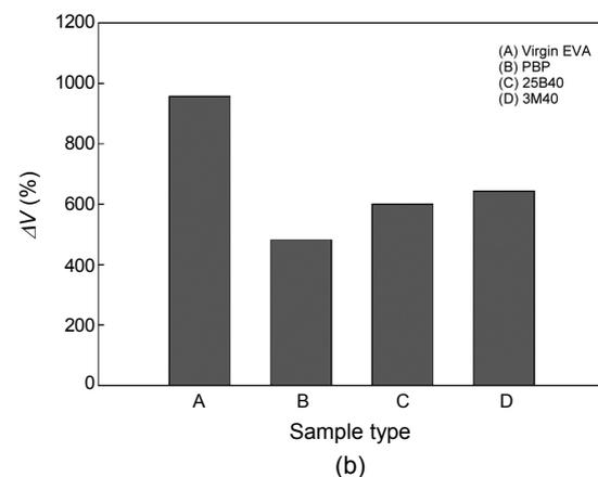
Figure 5. Swelling ratio of crosslinked EVA(21%) by various peroxides (a) without crosslinking acceleration agent; (b) with crosslinking acceleration agent.
