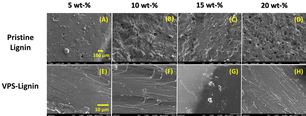
**Figure 5.** SEM micrographs of cryogenically fractured surface for the pristine Lignin/UPR (A-D) composite and VPS-Lignin/UPR composites (E-H).
