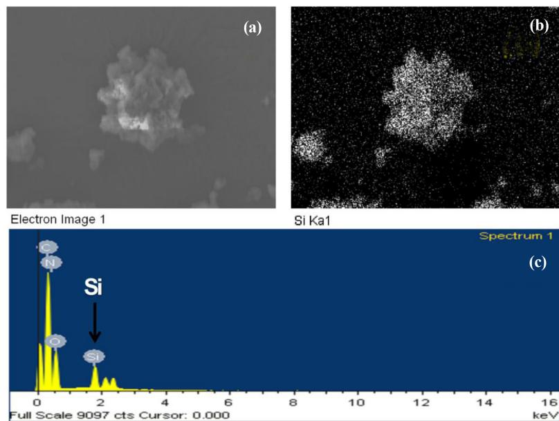
**Figure 2.** (a) SEM micrograph of the VPS-Lignin; (b) silicon element mapping image; (c) EDX spectrum of the VPS-Lignin.
