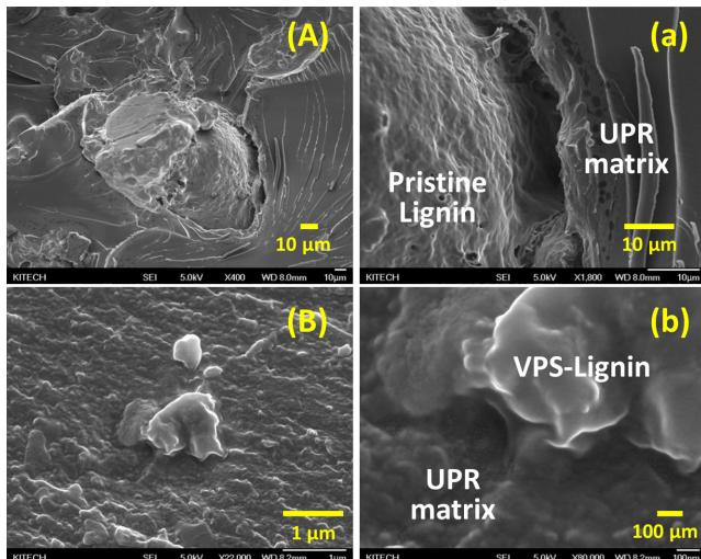
**Figure 6.** SEM micrographs and the magnified SEM micrographs of the pristine Lignin/UPR composite (A:a); VPS-Lignin/UPR composite (B:b).
