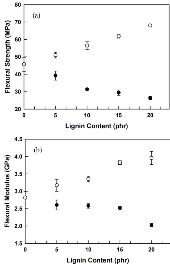
**Figure 3** Flexural strength (a); flexural modulus (b) of the pristine Lignin/UPR composites (●) and VPS-Lignin/UPR composites (○) according to Lignin content.
