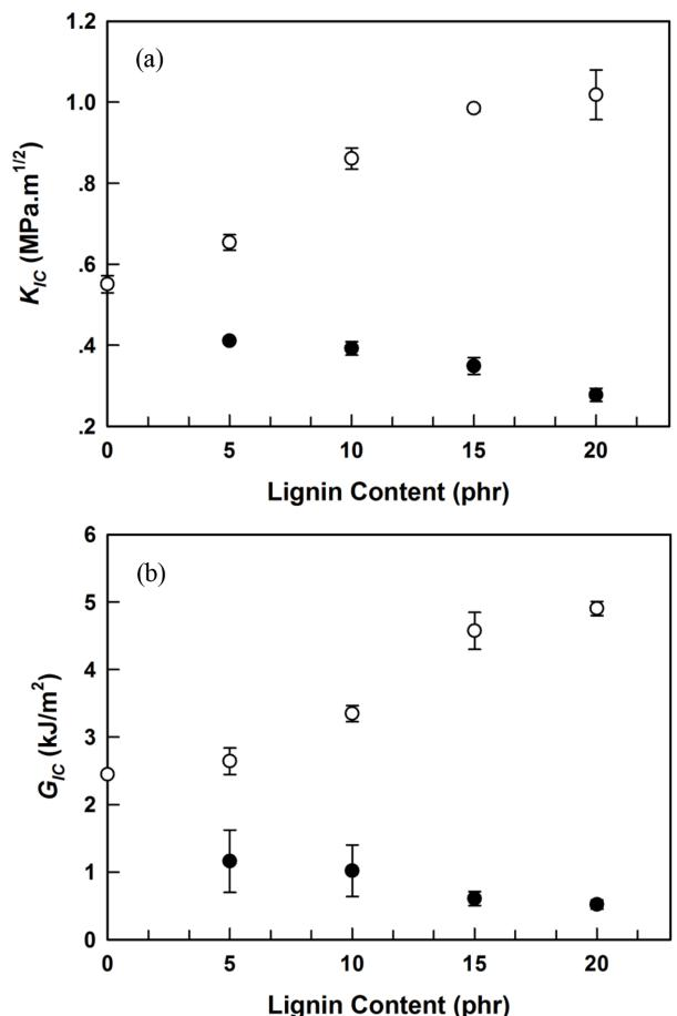
Figure 4. (a) Critical stress intensity factor ( $K_{IC}$ ); (b) critical strain energy release rate ( $G_{IC}$ ) of the pristine Lignin/UPR composites (●) and VPS-Lignin/UPR composites (○) according to Lignin content.
