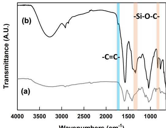
**Figure 1.** FTIR spectra of the pristine Lignin (a); VPS-Lignin (b).
