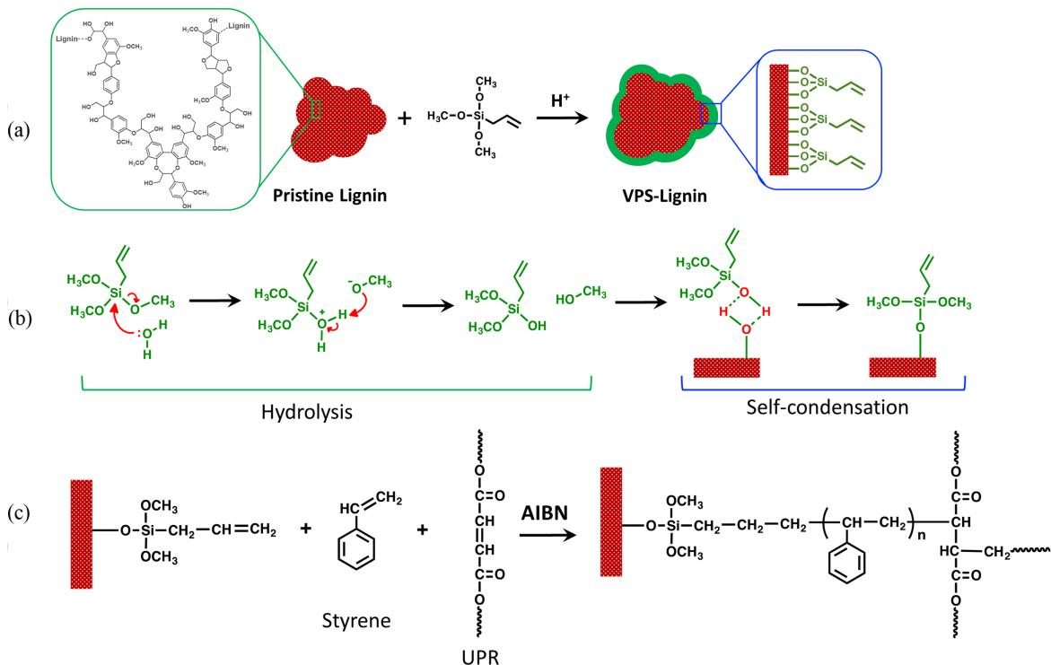
**Scheme 1.** Preparation outline of Lignin/UPR composite: (a) schematic outline for lignin modification; (b) hydrolysis-condensation mechanism; (c) schematic outline for UPR composite curing.
