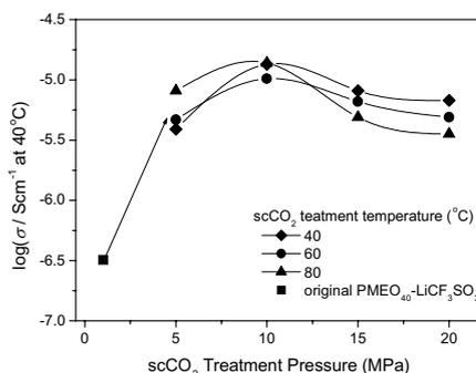
**Figure 5.** The effect of the treatment condition on the ionic conductivity at 40 °C for the original PMEО<sub>40</sub>-LiCF<sub>3</sub>SO<sub>3</sub> (■) and the scCO<sub>2</sub> treated samples (treatment temperature, 40 °C; ◆, 60 °C; ●, 80 °C; ▲).
