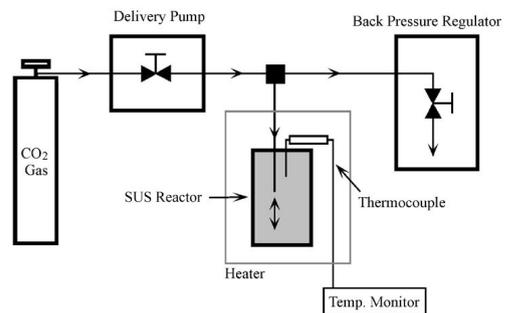
Figure 1. Schematic of experimental scCO<sub>2</sub> treatment setup.
