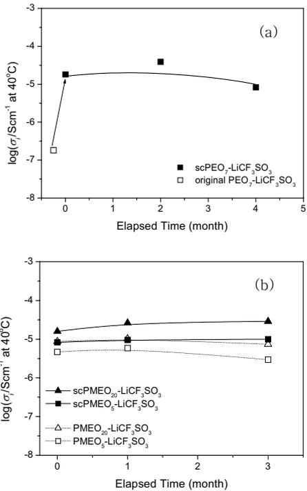
**Figure 7.** Time-dependence of the ionic conductivity at 40 °C for PEO-LiCF<sub>3</sub>SO<sub>3</sub> (a) and PMEО-LiCF<sub>3</sub>SO<sub>3</sub> (b).
