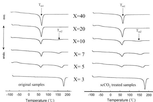
**Figure 4.** DSC thermograms of the original and the scCO<sub>2</sub> treated samples (PEO-LiCF<sub>3</sub>SO<sub>3</sub>).
