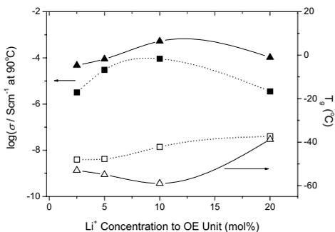
**Figure 6.** The effect of salt concentration on the ionic conductivity at 90 °C and  $T_g$  for the original PMEО-LiCF<sub>3</sub>SO<sub>3</sub> (■,▲) and the scCO<sub>2</sub> treated samples (□,△).
