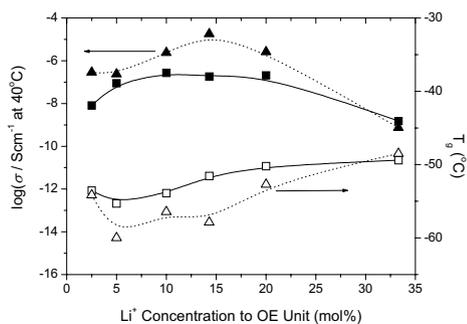
**Figure 3.** The effect of salt concentration on the ionic conductivity at 40 °C and  $T_g$  for the original PEO-LiCF<sub>3</sub>SO<sub>3</sub> (■, □) and the scCO<sub>2</sub> treated samples (▲, △).
