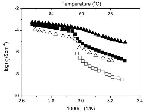
**Figure 2.** Temperature dependence of the ionic conductivity for the original PEO<sub>x</sub>-LiCF<sub>3</sub>SO<sub>3</sub> (□:x=40, △:x=7) and the scCO<sub>2</sub> treated samples (■:x=40, ▲:x=7).
