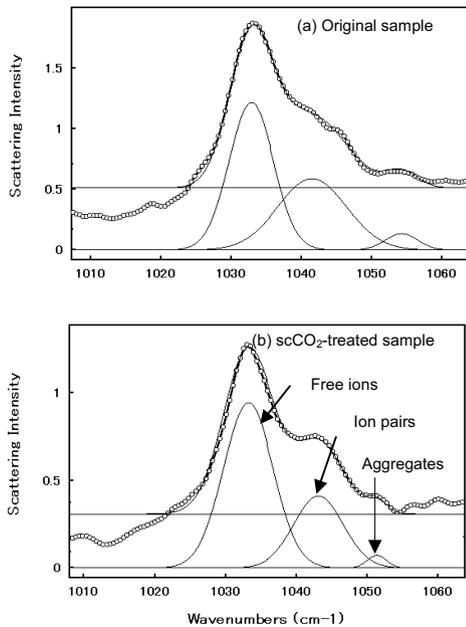
**Figure 8.** Raman spectrums of the original and scCO<sub>2</sub> treated samples: (a) original PMEO<sub>x</sub>-LiCF<sub>3</sub>SO<sub>3</sub> and (b) scPMEO<sub>x</sub>-LiCF<sub>3</sub>SO<sub>3</sub> (x=10, treatment condition: 40 °C, 10 MPa).
