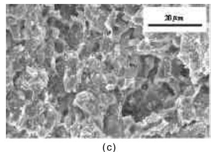
**Figure 2.** SEM micrographs of RPVC/RPE blends with different compositions. (a) RPVC/RPE 15/85, (b) RPVC/RPE 50/50, and (c) RPVC/RPE 85/15.
