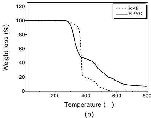
**Figure 1.** (a) DSC curves and (b) TGA curves of RPVC and RPE.
